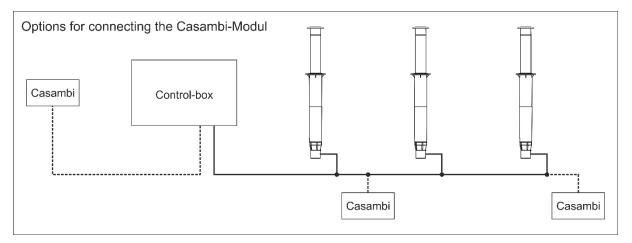
The Casambi module can be connected either to a separate, at least 2-wire cable directly on the control box, or alternatively to the DA+ and GND cable at any point of the main line to the luminaires.
