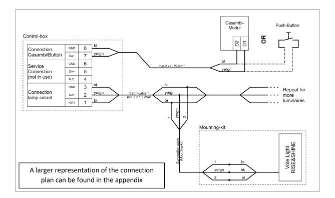
Optionally, a cable for the Casambi module can also be installed here.
