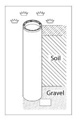
After aligning the mounting kit, fill it with about 10 cm of gravel. Fill the rest of the hole with soil up to about 20 cm below the upper edge and compact it with the help of a rod or similar.
